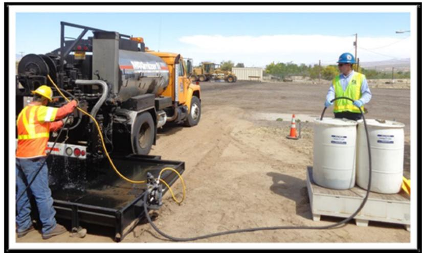
ADOT's internationally recognized Green Shop Program created spray guards for the agency's boot trucks in order to minimize environmental impact, reduce waste, and prevent equipment damage.
